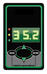
STEP 1 Press and hold the ENTER button, tS is displayed on the LEDs
